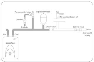
Kit contains - Expansion vessel, check valve (one way).
