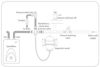
**Kit contains** - Manifold inc. check and service valve, pressure reducing valve, expansion vessel and bracket, flexible hose, tundish, 1/2" to 15 mm adaptor,  $3 \times 1/2$ " black rubber washers.
