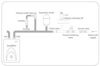
**Kit contains** - Expansion vessel, check valve (one way), pressure reducing valve.
