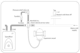
**Kit contains** - Manifold inc. check and service valve, expansion vessel and bracket, flexible hose, tundish, 1/2" to 15 mm adaptor,  $3 \times 1/2$ " black rubber washers.
