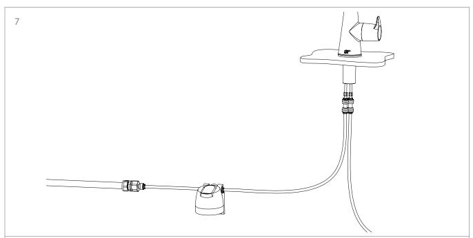
Calculate and cut the remaining section of  $\frac{1}{4}$ " tubing and make the final connections between fittings as per step 6. The remaining tap inlet should facilitate connection to the second cold drinking water selection. If this is unfiltered cold (ambient) follow steps above without a filter in the  $\frac{1}{4}$ " tubing. If chilled water is required follow separate chiller instructions.
