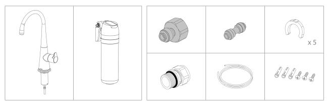
The required hole diameter is 32 mm. Can be installed onto a sink/ countertop up to 50 mm thick. Distance between centres - tap base to spout is 140 mm. Ensure this meets installation requirements.
