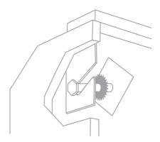
3 Choose the final mounting position of the heater. Consider the orientation required for the heater to ensure it will adhere to all previous warnings.
