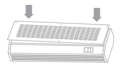
2 Loosen the bolts retaining the bracket inside the heater and remove the bracket from the heater completely.
