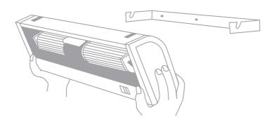
5 Offer up the heater to the bracket and locate the mounting bolts into the bracket lugs. Tighten the lugs enough to aid the orientation of the heater before tightening them firmly to prevent any future movement. Finally replace the air inlet cover on the front of the heater.
