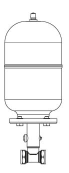
Assemble the vessel, t - piece and flow through valve as shown in figure 1.
