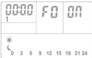
ON (open window detection on)
