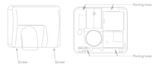
• Use the four screws provided to screw the back plate firmly to the wall.
