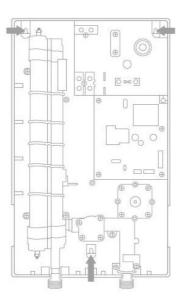
• Before attaching the appliance to the wall, consider the wiring route to the appliance. The electrical cable can enter through the opening in the back for concealed cabling. Knock out panels in the top right hand corner of the back plate and front cover are available for side entry.
