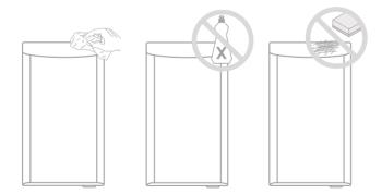
• Periodically remove any fluff, dust or lint etc. from the inside of the dryer. To do this first remove the cover and then, using a soft brush or vacuum cleaner, carefully remove any debris that exists.
